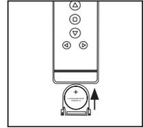
Insert the new battery (CR2430 lithium) into the battery tray so that the writing is facing up (positive up) when the remote is face up. Slide the tray back into the remote.
