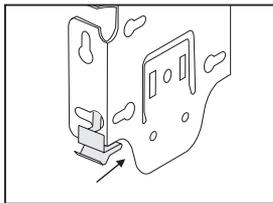
First, hook the fascia on the top of the bracket and then rotate downward.
