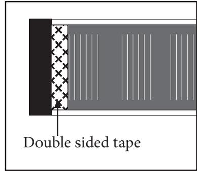
Clean the window surface with rubbing alcohol. When dry, remove the release liners and attach the solar panel to the glass, pressing firmly to adhere.
