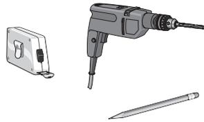
Additional fasteners other than those sent with your shade may be required depending on the mounting surface. Wallboard and plaster require the use of anchors such as expansion or toggle bolts. Brick, tile or stone need special plugs and drill bits. Remember to always pre-drill holes in wood to avoid splitting.
