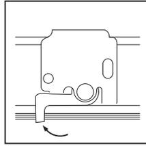
To attach the brackets the locking arm should be facing out. Then position the bracket so that it engages the inner front and inner back of the bracket, and then push the locking arm inward to lock it in place.
