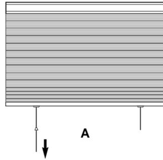
If the cord needs to be longer, slide the bottom end of the cord up into the plug and slide the plug down to take up slack.
