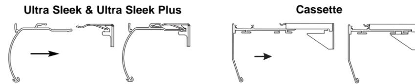
Push the rail back until it is fully engaged.
