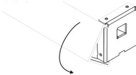
Swing the bottom of the fascia panel towards the bracket and gently press at the bottom of the panel until the lip on the fascia engages and snaps lock to the bracket.
