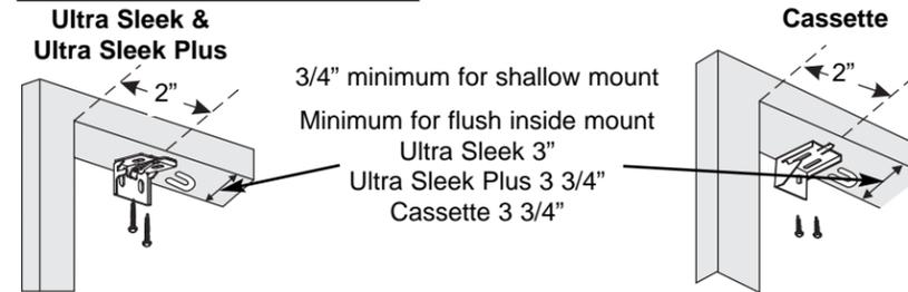
Use shims if necessary to ensure that the headrail is mounted level (included).
