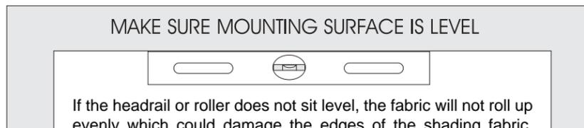
If the headrail or roller does not sit level, the fabric will not roll up evenly which could damage the edges of the shading fabric. Mount roller brackets as necessary, or use shims for headrail shades if necessary to level brackets.
