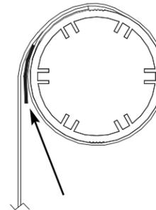
Roll the shade up and check for skewing. If the shade is still skewing, add another strip of tape on top of the first one. If the shade is now skewing to the opposite direction, tear off about 1" of tape from the last strip installed. The tape is to be torn from the end closest to the center of the shade.
