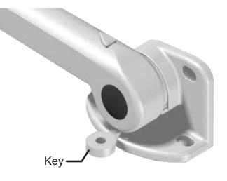
Hand Crank – Place hook of hand crank into the eyelet located at the bottom of the gear. Turn crank to extend the awning. Do not crank past the point of full extension, as fabric will slacken. Fabric must be retracted on the top of the roller tube, not the bottom.
