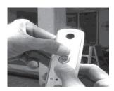
Press both the up and down button at the same time until the motor jogs.
